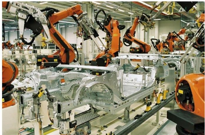
of industrial robots—computer-controlled machines used to perform repetitive tasks that are also hard or dangerous for human workers to perform.
