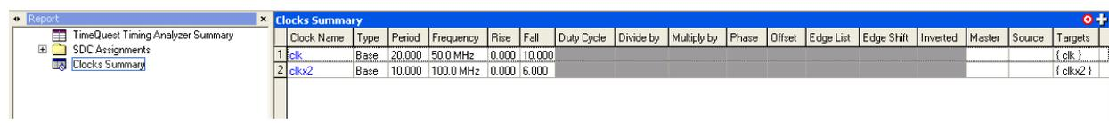
Use the **Report Clock Transfers** command to generate a report to verify that all clock-to-clock transfers are valid with the procedures in [Table 2-12](#). This report contains all clock-to-clock transfers in the design.
