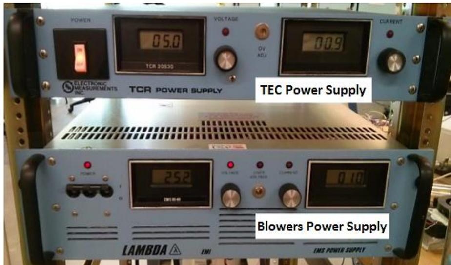
Figure 3.8 Test Stand power supplies.
