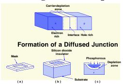
A *mask* is a specification of geometric shapes that need to be created on a certain layer. Masks are used to create a specific patterns of each material in a sequential manner and create a complex pattern of several layers
