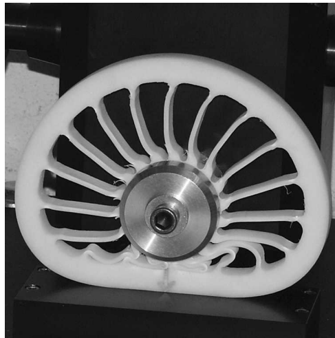
EXHIBIT 14-6 PackBot wheel prototypes (top) and impact testing (bottom).
