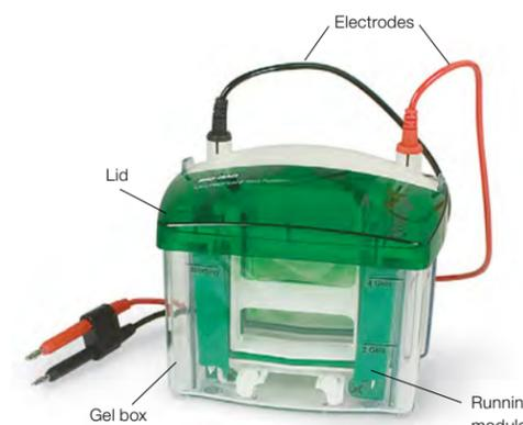
**Fig. 2.5. Components of a vertical electrophoresis cell.**
