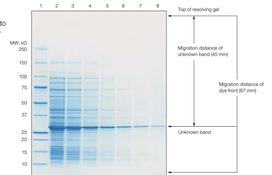
**Fig. 1. Example showing MW determination of an unknown protein.** Lane 1, 10 μl of Precision Plus Protein™ unstained standards; lanes 2–8, a dilution series of an *E. coli* lysate containing a hypothetical unknown protein (GFP). Proteins were separated by SDS-PAGE in a Criterion™ 4–20% Tris-HCl Gel and stained with Bio-Safe Coomassie stain. Gel shown is the actual size.
