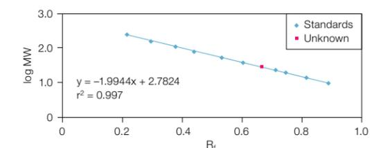
**Fig. 2. Determining the MW of an unknown protein by SDS-PAGE.** A standard curve of the log (MW) versus R<sub>f</sub> was generated using the Precision Plus Protein standards from Figure 1. The strong linear relationship ( $r^2 > 0.99$ ) between the proteins' MW and migration distances demonstrates exceptional reliability in predicting MW.
