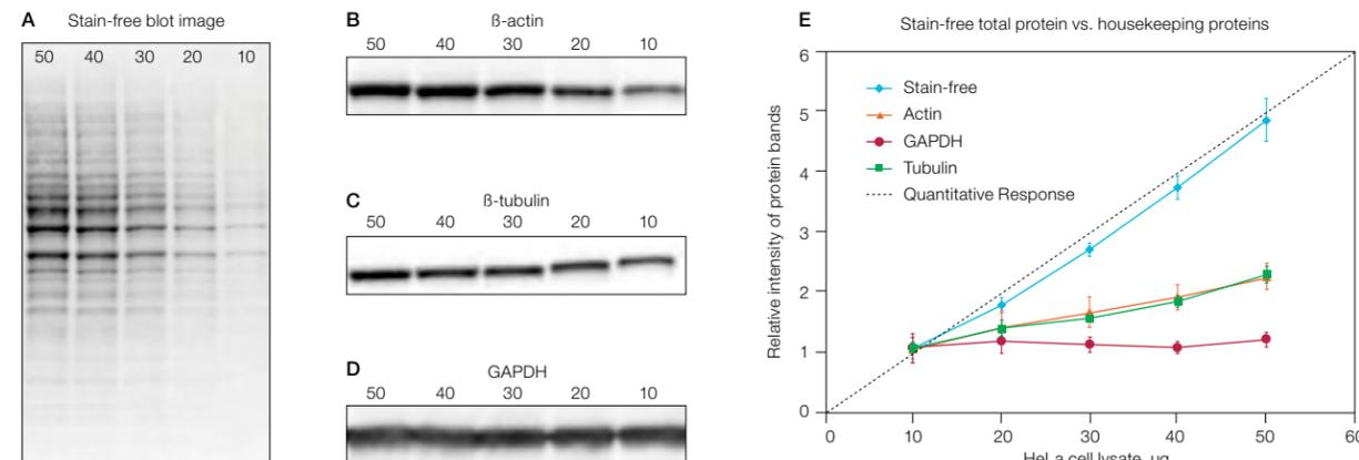
Fig. 6.4. Comparison of protein normalization using stain-free technology and commonly used housekeeping proteins. Tenfold dilutions of HeLa cell lysates ranging from 50 to 10  $\mu$ g were loaded for samples detected with stain-free technology (A) and the housekeeping genes  $\beta$ -actin (B),  $\beta$ -tubulin (C), and GAPDH (D). The protein quantification signal is higher with stain-free technology than with housekeeping genes (E).
