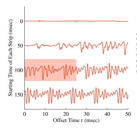
A microphone has converted the sound pressure from the vocal tract into an electrical signal that varies over time, *t*
