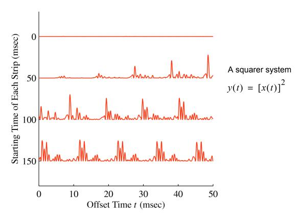
• The squarer system also exists for discrete-time signals, and in fact is easier to implement, since all we need to do is multiply each signal sample by itself
