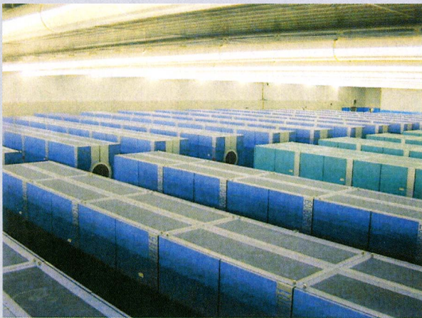
FIG. SBI. The Earth Simulator machine of the Frontier Research Project. The machine is located in Yokohama, Japan. Its measured performance is 35.61 Tflops. It consists of 640 nodes that are connected by a high-speed network. Each node contains eight vector processors with 16 GB of memory, for a total of 5120 processors and 10 TB of memory. The Earth Simulator is capable of running a super-GCM fast enough to enable practical climate change simulations.
