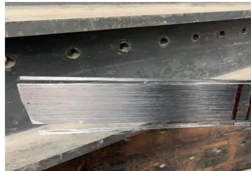
**Figure 10.** Carbon plate longitudinal splitting failure
