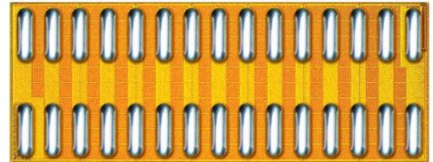
Figure 7: Fourth generation eGaN devices had lower on-resistance and better switching figures of merit. This EPC2023 has a 30 V, 1.3 mΩ rating and can handle 590 A pulsed.
