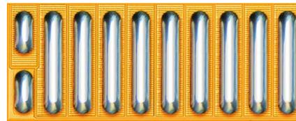
Figure 1: The EPC1001 was first launched in March 2010. It had a maximum on-resistance of 7 mΩ and a voltage rating of 100 V.
