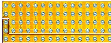
Figure 8: The first GaN-on-Si power integrated circuit was a monolithic half bridge such as the EPC2101 pictured above.
