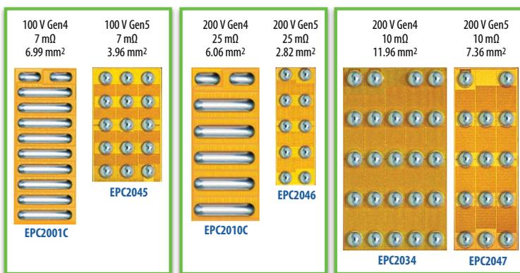
Figure 1: EPC's fifth-generation technology cuts the die size in half for the same on-resistance and voltage rating
