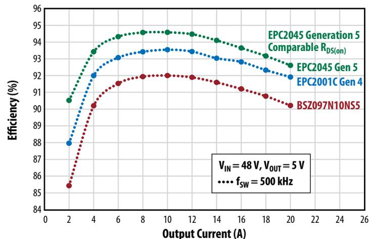
Figure 3: Gen 5 Devices have higher performance and are about half the size of Gen 4. Both Gen 5 and Gen 4 are far superior to the best available MOSFET.
