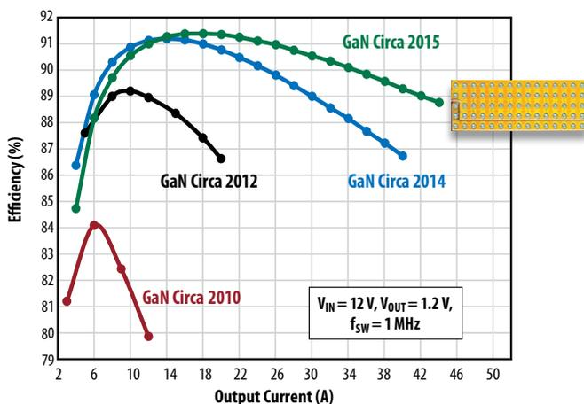
Figure 9: EPC has continuously improved eGaN technology as demonstrated by the continued gains in efficiency in a 12 V – 1 V buck converter operating at 1 MHz. The most efficient system (GaN circa 2015) uses a monolithic half bridge.
