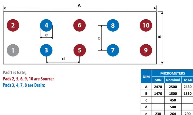
Figure 7: The pitch of 200 V Gen 5 transistors is the same as Gen 4 200 V at 600 μm.
