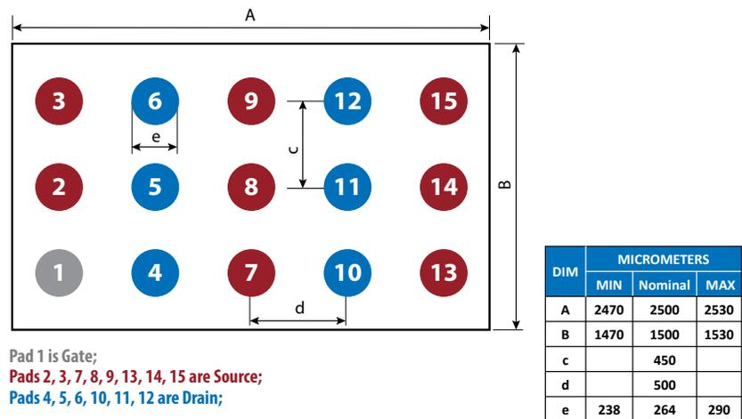
Figure 6: In comparison to Gen 4 devices, the pitch of 100 V Gen 5 transistors has been increased to 450 μm.
