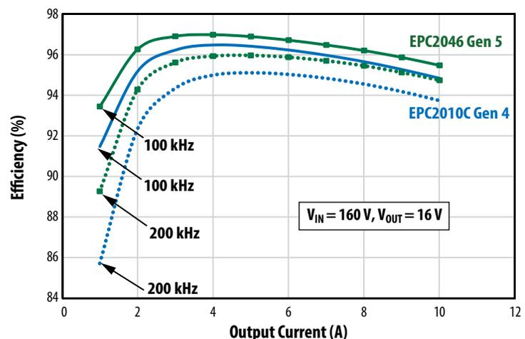
Figure 4: Comparison of efficiency of 200 V eGaN FETs from Gen 4 and Gen 5 at 100 kHz and 200 kHz. Despite being half the size and having the same on-resistance and voltage rating, the Gen 5 devices outperform Gen 4 by a wide margin.
