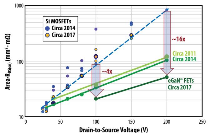
Figure 2: EPC's fifth-generation technology cuts the die size in half for the same on-resistance and voltage rating. At 200 V the eGaN FET die size is more than 16 times smaller than an equivalently-rated silicon MOSFET.
