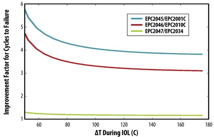
Figure 5. Shown is the relative power cycling performance of Gen 5 devices compared with Gen 4. Smaller die sizes have less differential thermal expansion with the underlying PCB, thus reducing strain during thermo-mechanical cycling.
