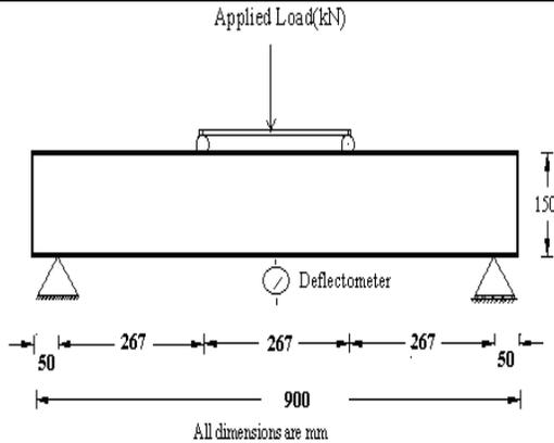
Figure 1: Details of test beams
