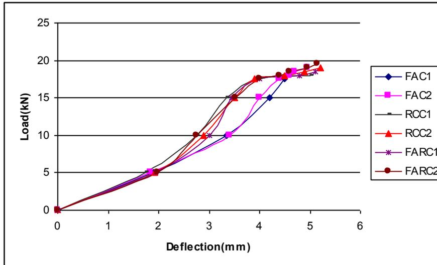
Figure 3: Relation between Load and Deflection of Beams
