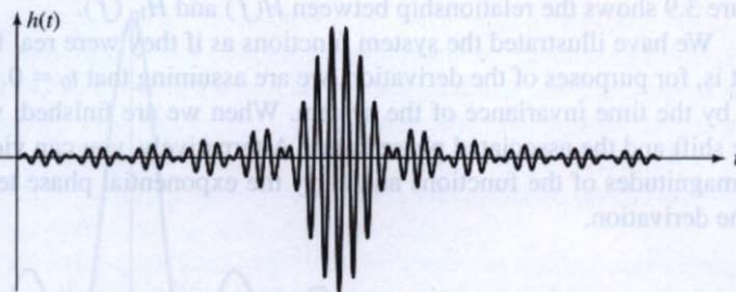
Figure 3.10 Impulse response of ideal bandpass filter.
