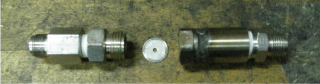
**Figure 3.5 – Orifice plate flow restrictor.**
