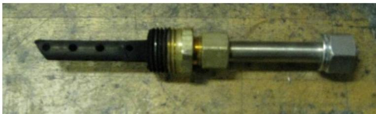
**Figure 3.7 – Sampling probe.**
