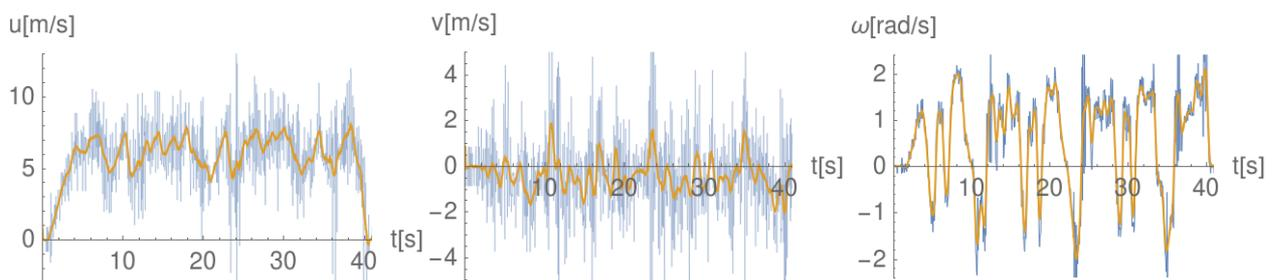
**Figure:** Discrete differences yield the tangent velocity  $u$ , side-slip velocity  $v$ , and heading rate  $\omega$  before (blue) and after smoothing (yellow).
