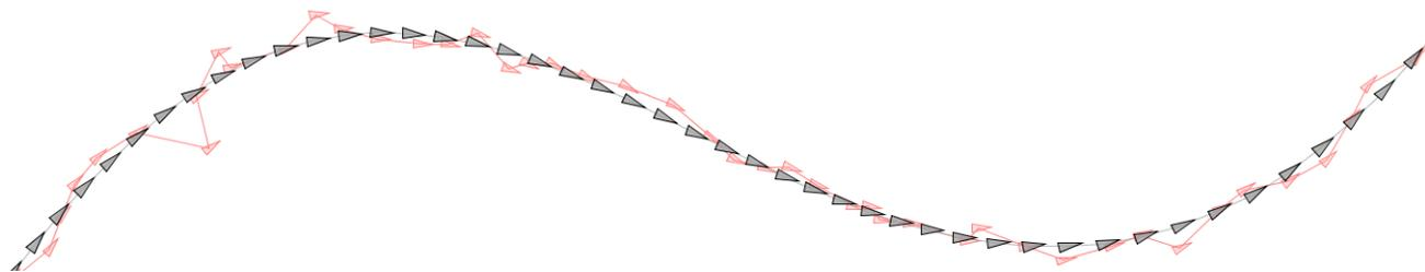
**Figure:** A sequence of noisy localization estimates of a fast driving go-kart in red, and the result of smoothing in black. ■
