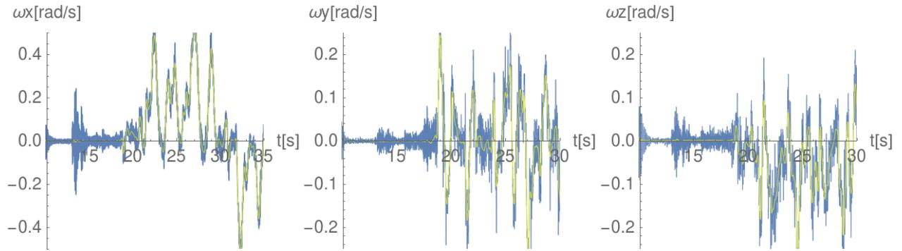
**Figure:** The orientation components of the discrete differences before (blue) and after the smoothing (yellow) during the time 10 – 35[s]. ■
