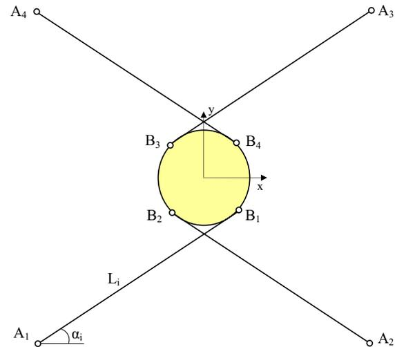
Fig. 1. The schematics of a 4RPR planar cable driven redundant parallel manipulator
