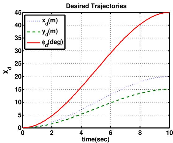
Fig. 3. Desired Trajectory devised for the Planar CDRPM
