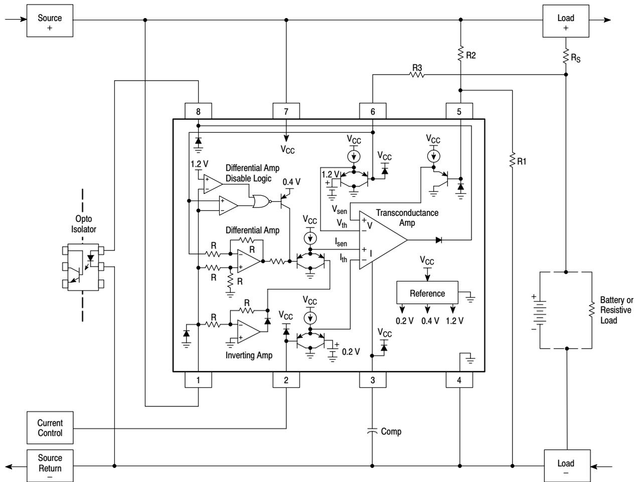
The above figure shows the MC33341 configured for load high-side current sensing with an externally adjustable current threshold. Operation of this circuit is similar to that of Figure 17. The current regulation threshold can be adjusted over a range of 0 V to 200 mV with respect to Pin 4.
