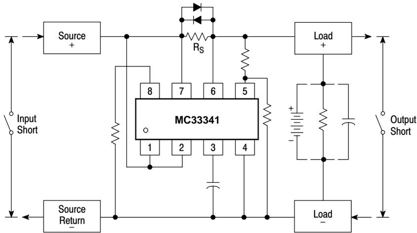
**NOTE:** An excessive load induced voltage across  $R_S$  can occur if either the source input or load output is shorted. This voltage can easily be bounded with the addition of the diodes shown without degrading the current sensing accuracy. This bounding technique can be used in any of the MC33341 applications where high peak currents are anticipated.
