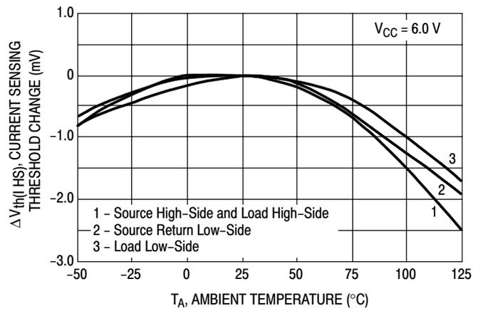
**Figure 2. Current Sensing Threshold Change versus Temperature**
