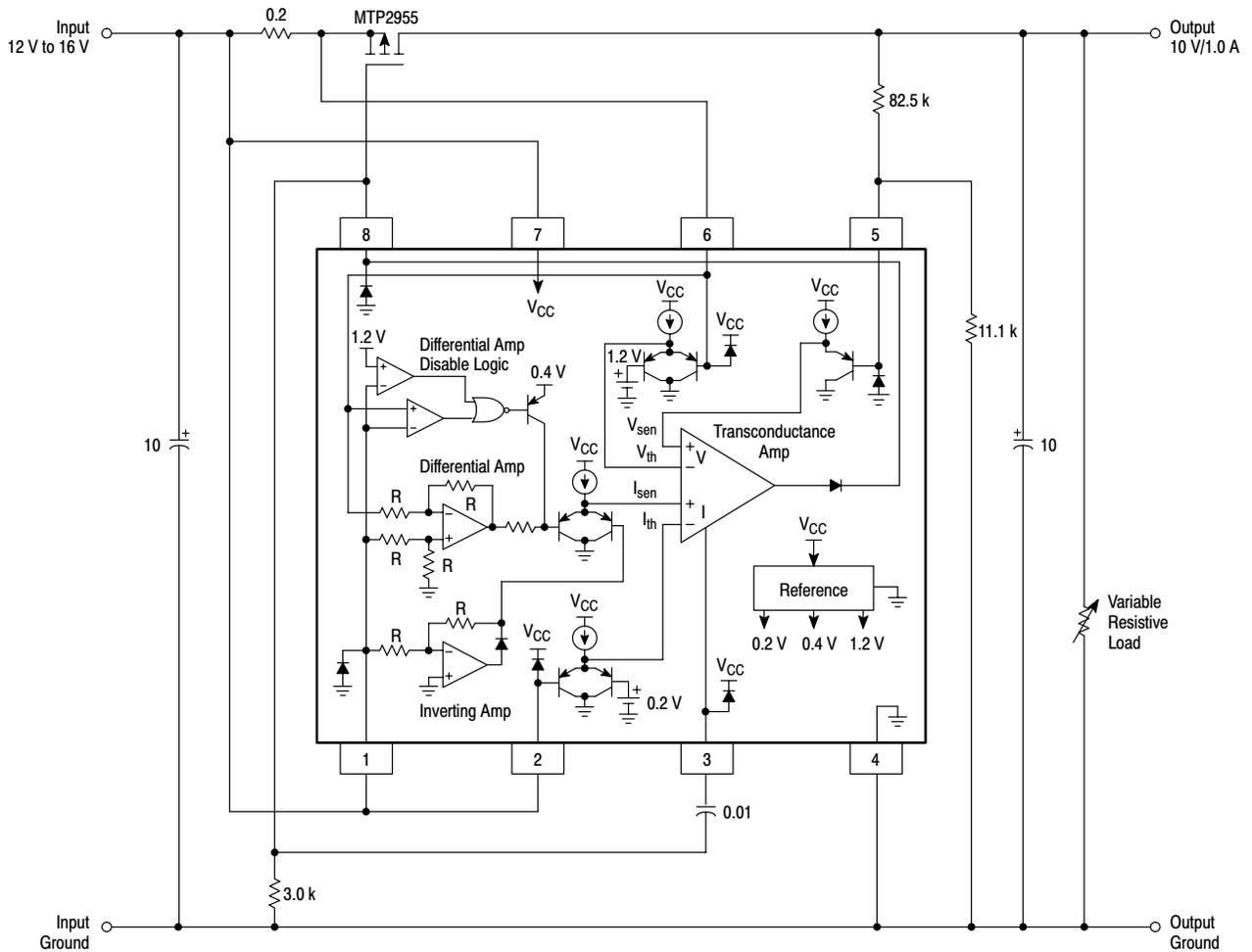
Figure 23. 10 V/1.0 A Constant-Voltage Constant-Current Regulator
