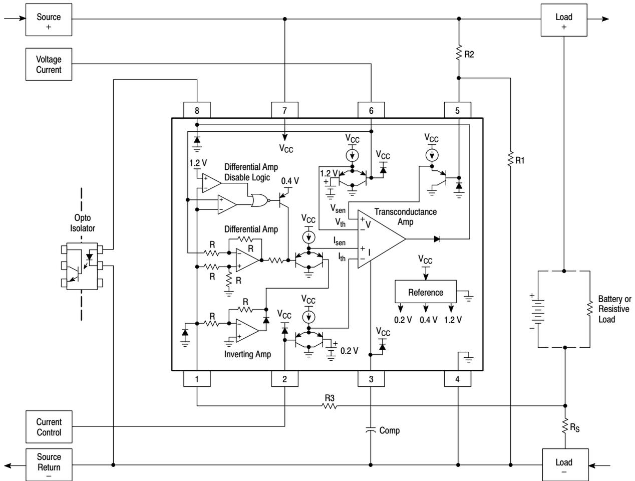
The above figure shows the MC33341 configured for load low-side current sensing with an externally adjustable voltage and current threshold. Operation of this circuit is similar to that of Figure 19. The respective voltage and current regulation threshold can be adjusted over a range of 0 to 1.2 V and 0 V to 200 mV, with respect to Pin 4.
