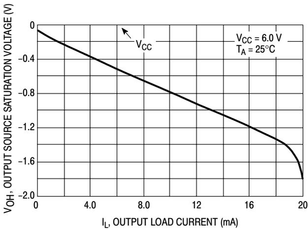
**Figure 11. Drive Output High State**
