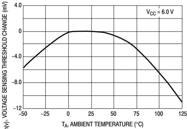
**Figure 1. Voltage Sensing Threshold Change versus Temperature**
