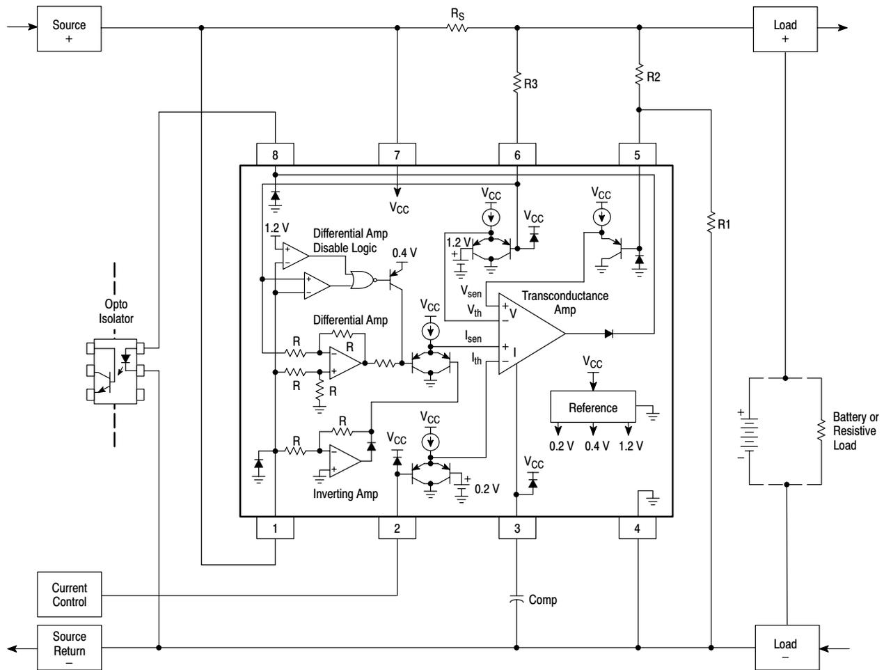
The above figure shows the MC33341 configured for source high-side current sensing with an externally adjustable current threshold. Operation of this circuit is similar to that of Figure 13. The current regulation threshold can be adjusted over a range of 0 V to 200 mV with respect to Pin 4.
