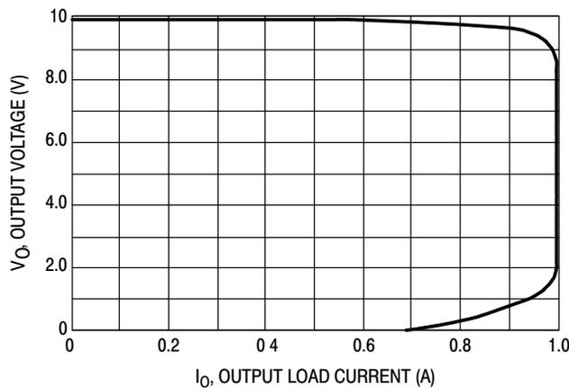
Figure 23 shows the MC33341 configured as a source high-side constant-voltage constant-current regulator. The regulator is designed for an output voltage of 10 V at 1.0 A. Figure 24 shows the regulator's output characteristics as the load is varied. Source return low-side, load high-side, and load low-side configurations will each exhibit a nearly identical load regulation characteristic. A heatsink is required for the MTP2955 series pass element.
