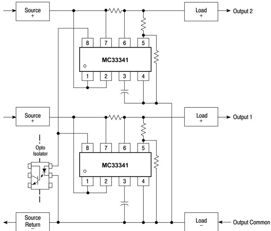
**NOTE:** Multiple outputs can be controlled by summing the error signal into a common optoisolator. The converter output with the largest voltage or current error will dominate control of the feedback loop.
