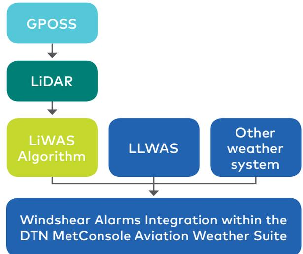
Diagram of interactions between the most relevant components of a LiWAS System.
