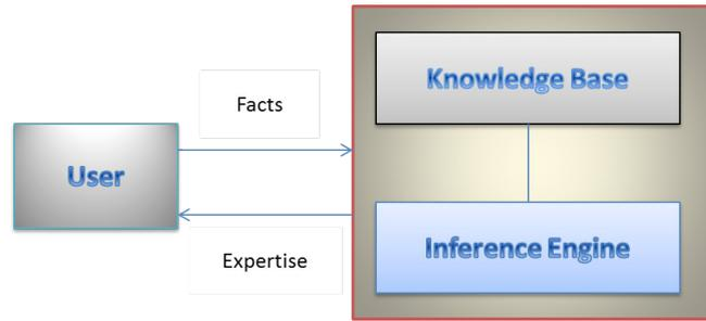
Figure 1 Main Components of an Expert System [11]
