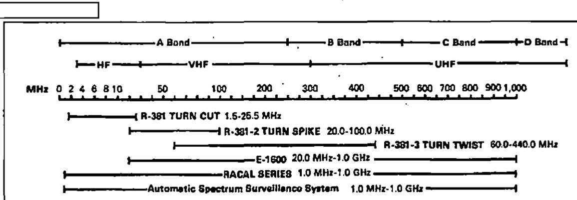
Figure 3. [ ] Iraq Electronic Support Measures Frequency Spectrum [ ]
