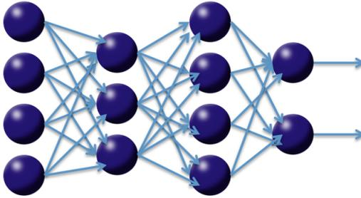
Bias units are included in each non-output layer of the network. The weights linking neurons and biases with other neurons fully determine the output of the entire network. Learning occurs when these weights are adapted to minimize the error on the labeled training data. More specifically, for each training example  $j$ , the objective is to minimize a loss function,
