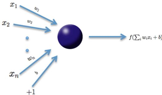
Multi-layer, feedforward neural networks consist of many layers of interconnected neuron units (as shown in the following image), starting with an input layer to match the feature space, followed by multiple layers of nonlinearity, and ending with a linear regression or classification layer to match the output space.
