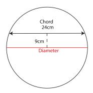
We can arrive at this diagram from the information given. We can find the radius by making a triangle with half the chord and the height 9cm.
