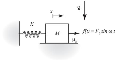
Figure 3. Simple Coulomb friction model.
