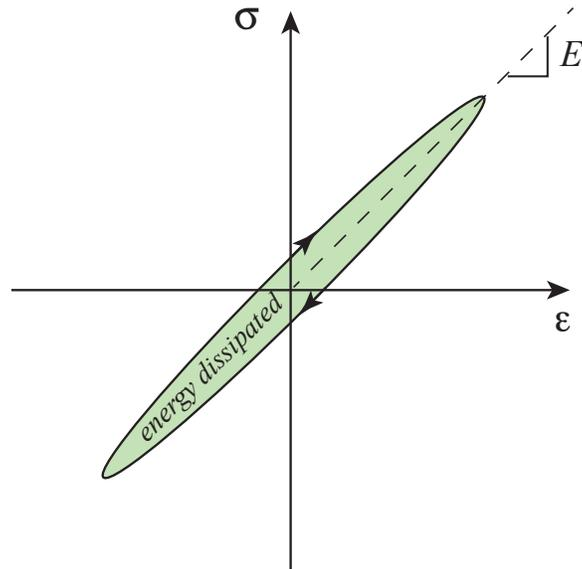
Figure 7. Stress-strain curve for hysteretic damping model.
