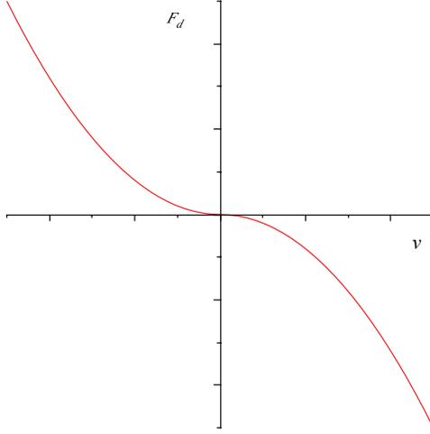
Figure 5. Force due to quadratic damping
