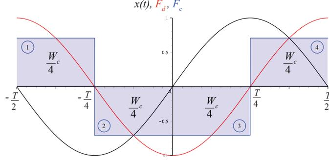
Figure 4. Normalized viscous and Coulomb friction resistance force, and displacement over one period.
