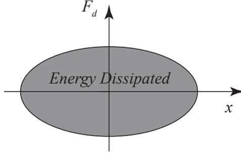
Figure 2. Viscous damper dissipated energy ellipse at resonance.
