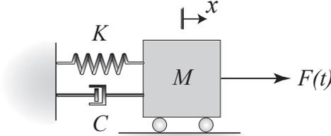
Figure 1. Forced mass-spring-damper system.
