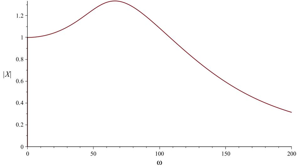
Figure 6. Amplitude of quadratically-damped harmonic response.
