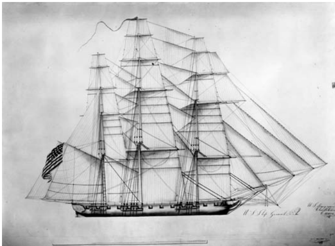
Fig 3.49: Spar and sail plan of the sloop General Pike , which served on Lake Ontario. (U.S. Naval Historical Center)
