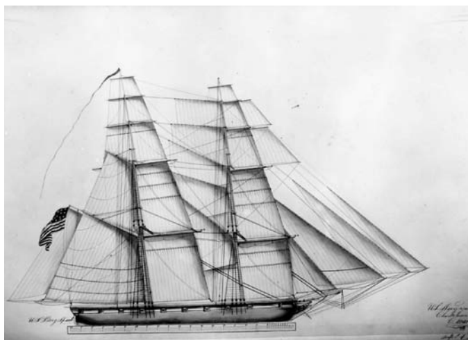
Fig 3.36: Spar and sail plan of the brig Spark , built in 1813 and purchased at New York. (U.S. Naval Historical Center)
