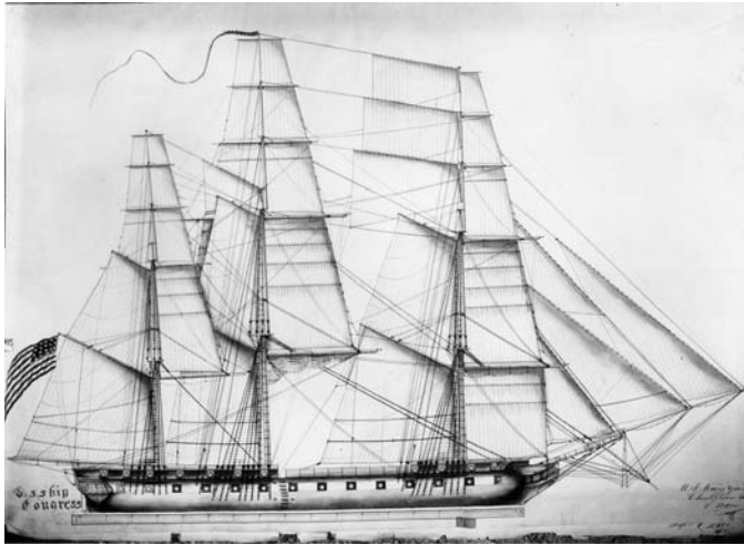
Fig 3.14: Spar and sail plan of the frigate Congress of 1799. (U.S. Naval Historical Center)
