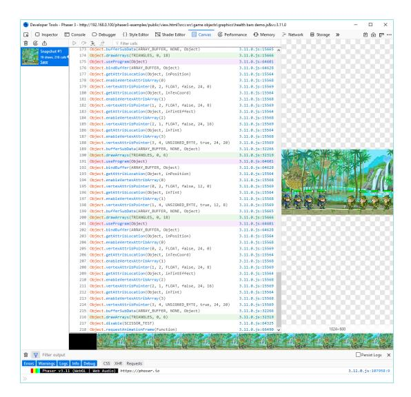
It's a little tricky to make out if you're looking at the image embeddd in the newsletter - but the important part is that this simple scene is using no less than 19 draw calls and a staggering 218 WebGL operations.
