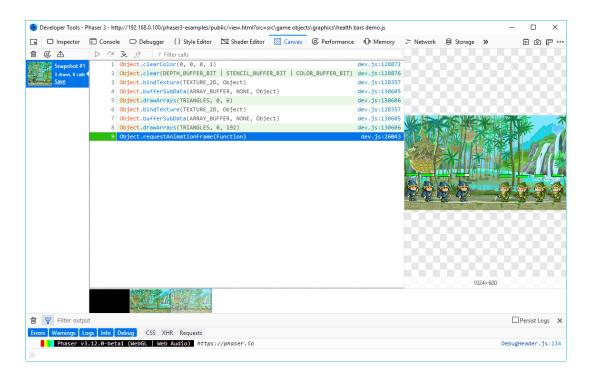
Again, it might be hard to tell from the size of the screen shot, but you should immediately see there are far less draws going on (the thumbnails along the bottom) and the list of gl ops is massively smaller:
