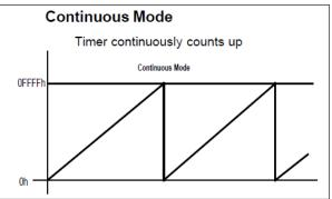
To add further functionality, there can be multiple CCR registers active at the same time, so the timer can generate interrupts at multiple custom time intervals within a larger period.
