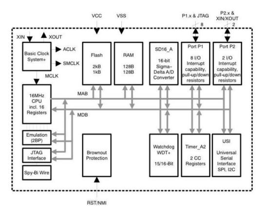
Apart from the 16MHz CPU, we can also see peripherals for communication, analog-to-digital conversion and timers. There are also general purpose digital pins which can also be utilized for interaction with external devices. This tutorial will subsequently go over each of the above mentioned components and more.
