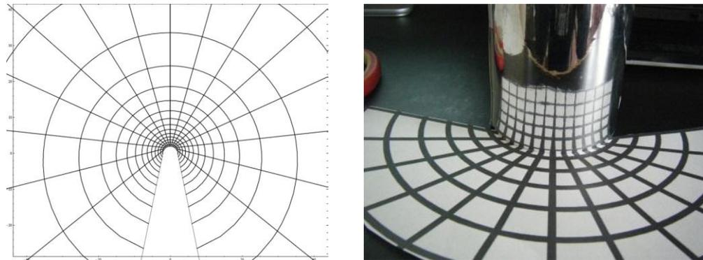
**Figure 1:** Transformation of a rectangular grid using the formulas found (left) with the cylinder reconstituting the image (right).
