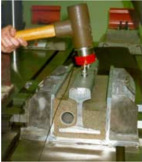
Figure 14.24: Recording properties of embedded rail test sample in laboratory
