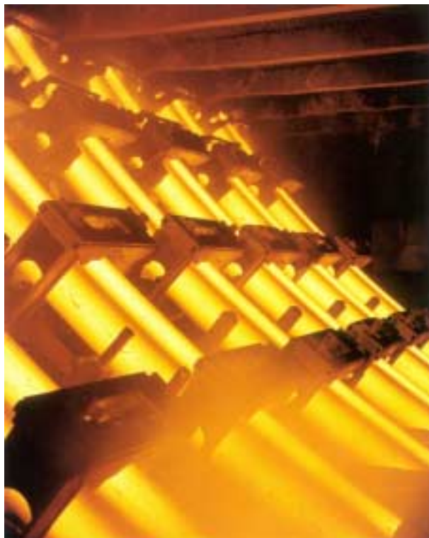
Figure 10.8: Hot strands passing through cooling chambers in a circular arc
