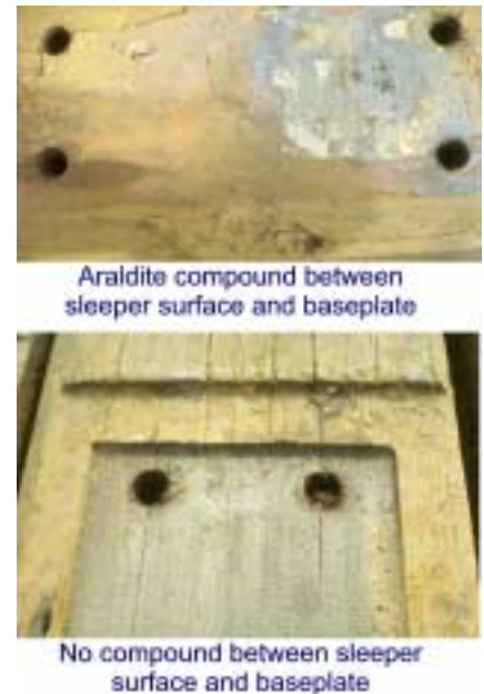
Figure 8.22: Effect of sleeper treatment with araldite
