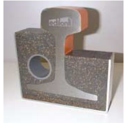
Figure 5.30: Standard UIC 54 Embedded Rail Structure
