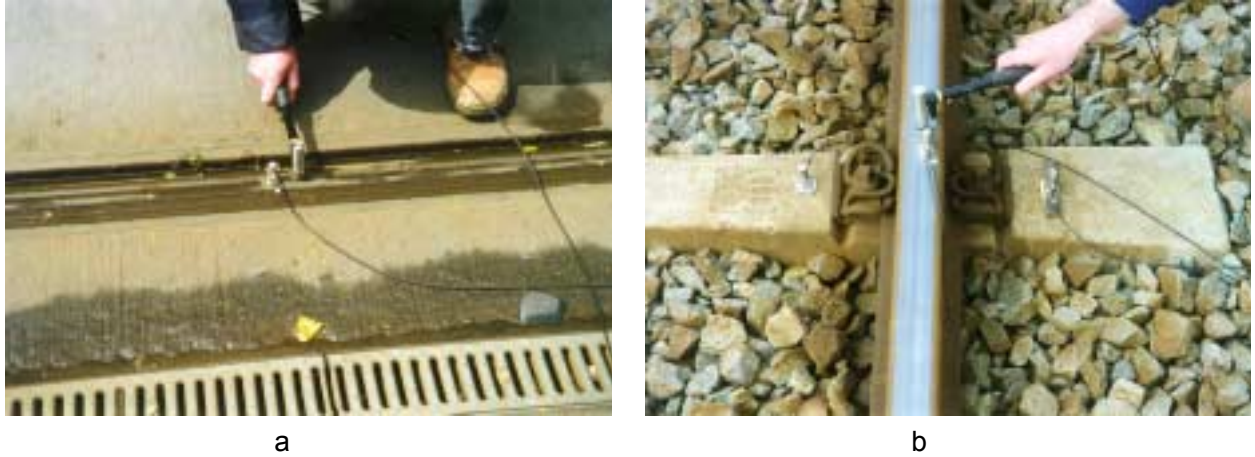
Figure 13.26: Hammer Excitation Test on classical track (a) and Embedded Rail Structure (b)
