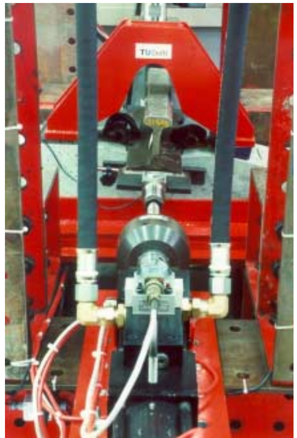
Figure 14.10: Longitudinal resistance test of a fastening system mounted on a sleeper
