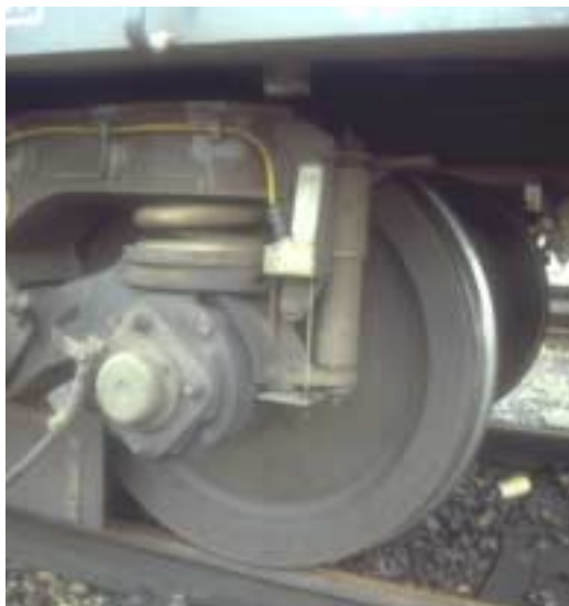
Figure 16.83: Transducer for vertical displacement between axle and bogie frame
