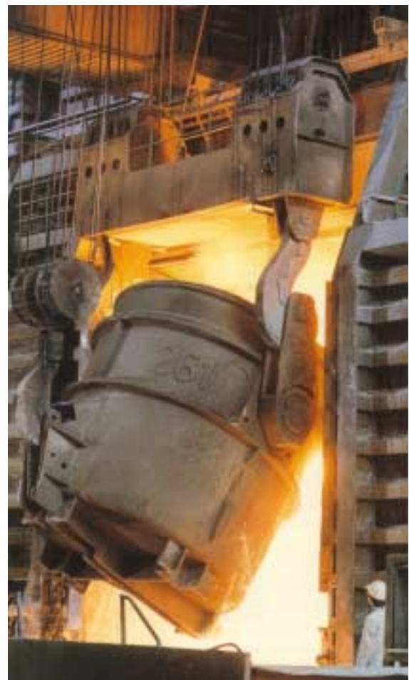
Figure 10.4: Filling proces of converter
