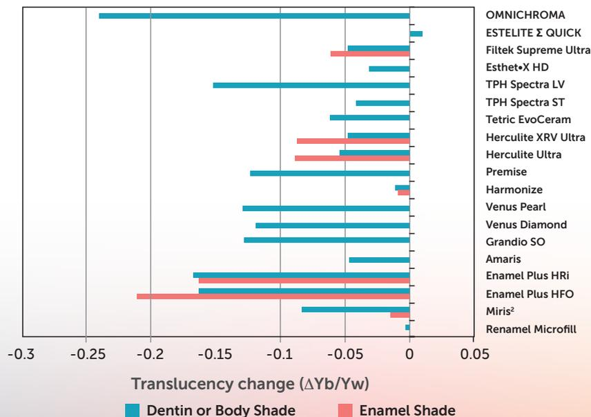
Fig. 29 Change of translucency before and after polymerization
