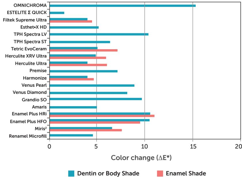
Fig. 28 Change of color before and after polymerization
