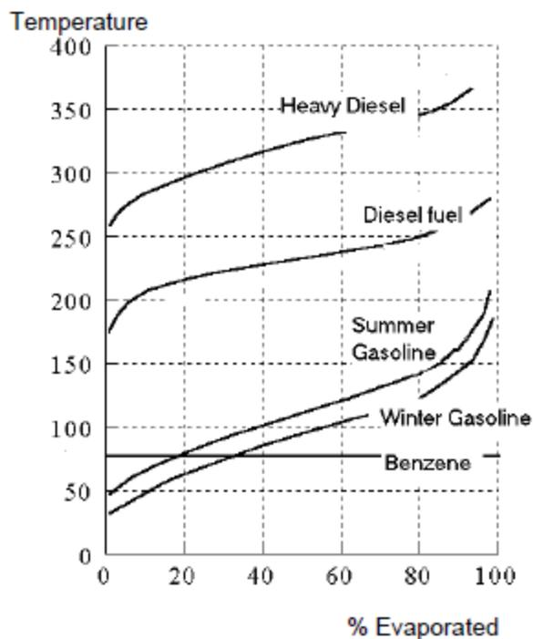
**Fig. 12. Distillation curve**
