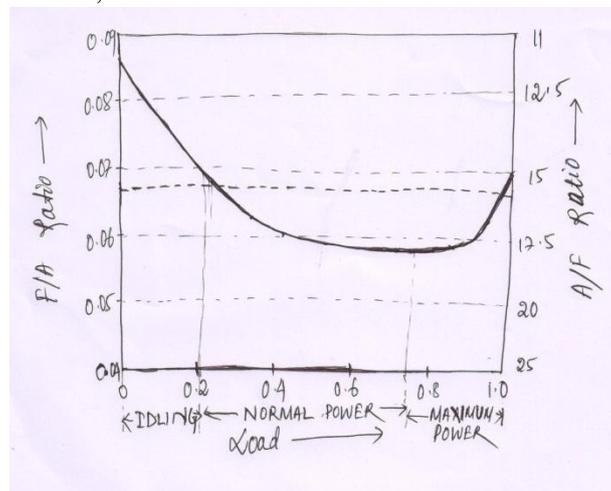
**Fig. 13. Main areas of automotive engine operation**
