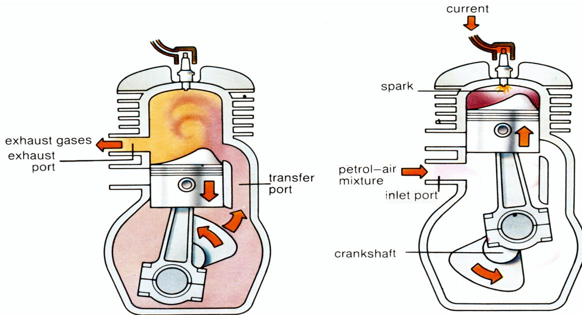
**Fig. 3.** Cycle of operation in two stroke engine
