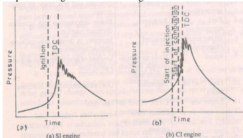
**Fig. 28. Detonation in SI and CI engine**
