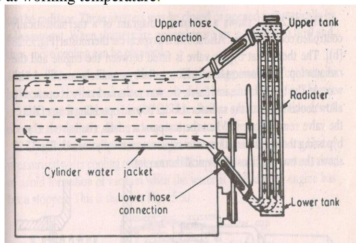
**Fig. 37. Thermo-syphon cooling**
