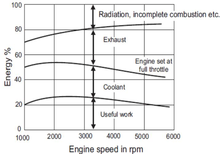
**Fig. 35. Heat balance sheet for SI engine**
