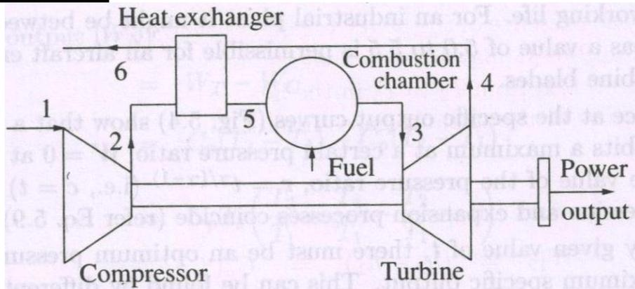
**Fig. 45. Simple gas turbine with heat exchanger**
