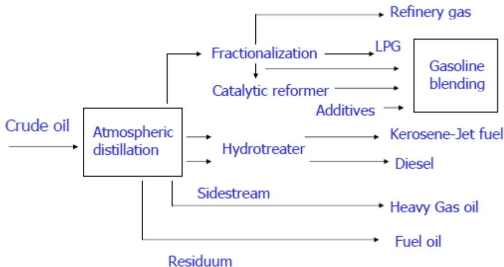
**Fig. 10. Refinery processes**
