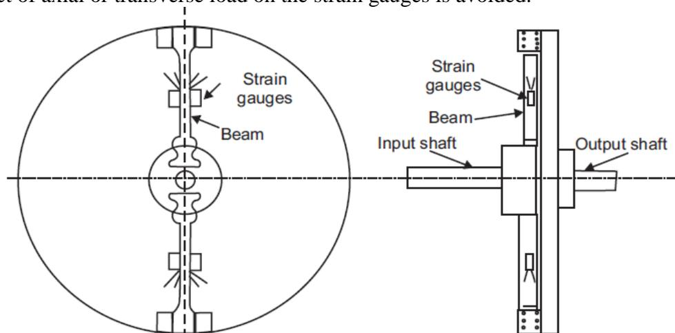
Fig. 33. Transmission dynamometer
