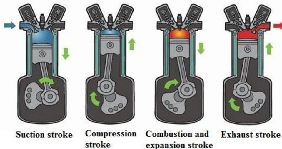
**Fig. 2.** Cycle of operation in four stroke engine
