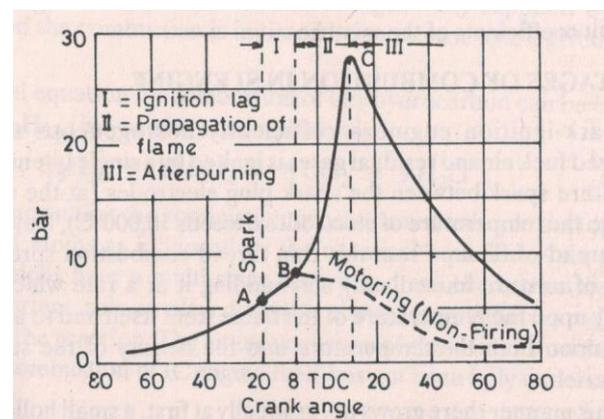
Fig. 25. Stages of combustion in SI engine
