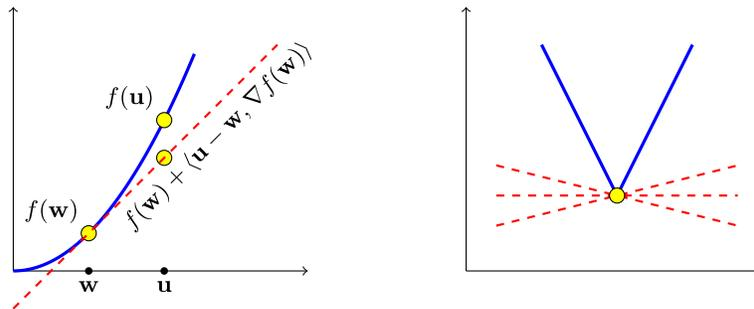
Fig. 2.1 Left: The right-hand side of Equation (2.3) is the tangent of  $f$  at  $\mathbf{w}$ . For a convex function, the tangent lower bounds  $f$ . Right: Illustration of several sub-gradients of a non-differentiable convex function.
