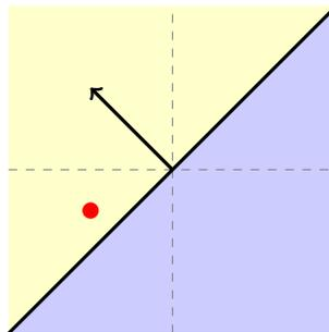
Fig. 3.3 An illustration of linear separators in the plane ( $\mathbb{R}^2$ ). The *solid black line* separates the plane into two regions. The *circled point* represents an input vector which is labeled 1 by the linear separator. The arrow designates a weight vector that represents the hypothesis.
