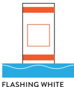
**Mooring Buoys** – Buoys designed for mooring boats are all-white with a blue stripe midway between the top and the waterline. A minimum of 16 square inches of white reflector, part of which must be visible from any direction, is required on all mooring buoys. (Obtain a permit from the county sheriff before placing a mooring buoy in the water.)
