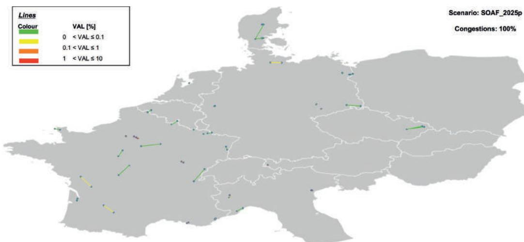
Figure 4.27: All N-0 grid constraints that have a non-zero shadow price for at least one hour in the SOAF 2025 worst case scenario, coloured by weight of the constraint in the congestion costs – based on the assumption of an only partial implementation of the planned network extensions
