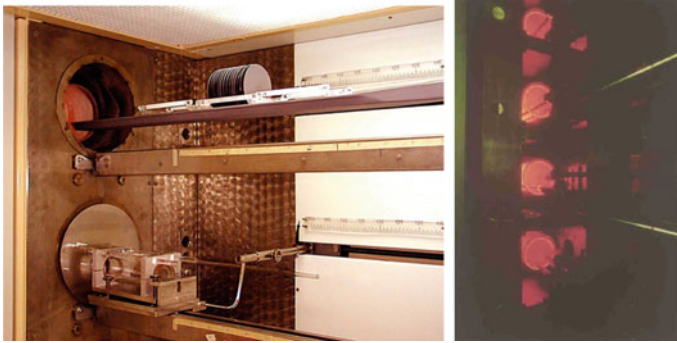
Fig. 1.53 Two quartz tubes in the furnace are visible on the left photo including the loader of several wafers. Each individual furnace has a well-defined atmosphere and always remains at the same temperature and content mixture. There is one furnace for each individual process. On the right , several burning furnaces are shown. Courtesy of ITE Warsaw [347]
