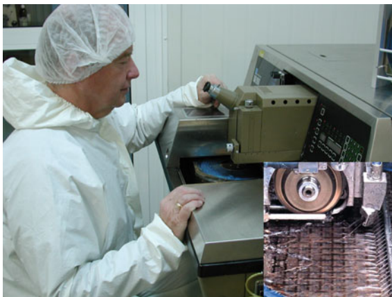
Fig. 1.65 The cutting of chips with a diamond saw. Note the high water flux to avoid heating up due to the high saw rotation speed. Courtesy of ITE Warsaw [347]
