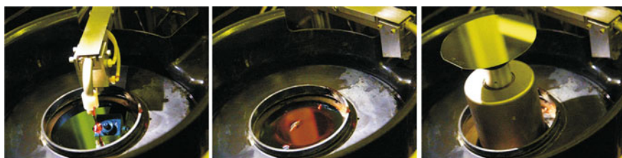
Fig. 1.55 Photoresist is roughly spilled in the middle of the wafer, centrifugal forces, during fast rotation, homogeneously distributes the resist on the wafer. Courtesy of ITE Warsaw [347]
