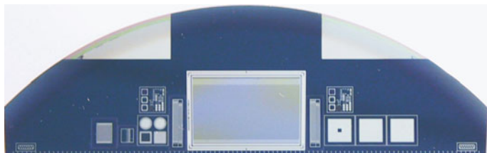
Fig. 1.45 Half-moon with test structures. Left to right , the structures with the following accessible process parameter are located (1) TS-CAP ( C_{\text{coupling}} , V_{\text{break}} ). (2) sheet (Resistivity Al , Resistivity p+ , R_{\text{poly}} ). (3) Gate Controlled Diode GCD ( I_{\text{surface}} ). (4) CAP-TS-AC ( C_{\text{inter-strip}} ). (5) full minisensor. (6) CAP-TS-DC ( R_{\text{inter-strip}} ). (7) Diode ( V_{FD} ). (8) MOS1 ( V_{\text{flat-band}} ). (9) MOS2 ( V_{\text{flat-band}} )
