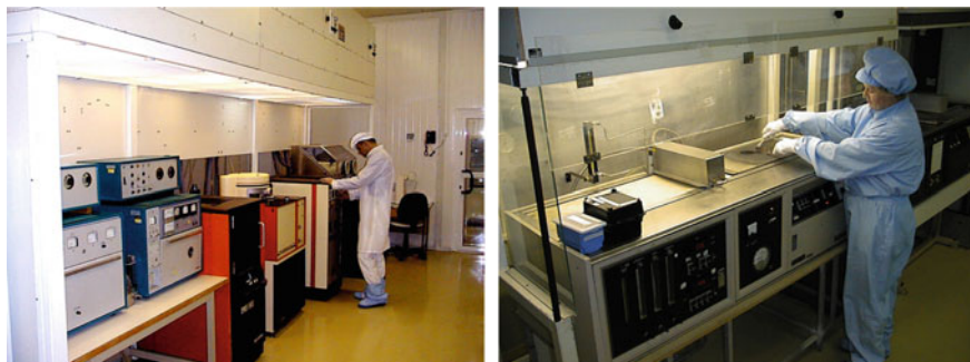
Fig. 1.57 On the left , the plasma etching laboratory of a silicon plant in an institute is shown. On the right , the wet etching facility is displayed. The secret and art lies in the special recipes to use the right acid, the right duration and time on the different structures and materials, like \text{Si} , \text{SiO}_2 and \text{Al} . Courtesy of ITE Warsaw [347]
