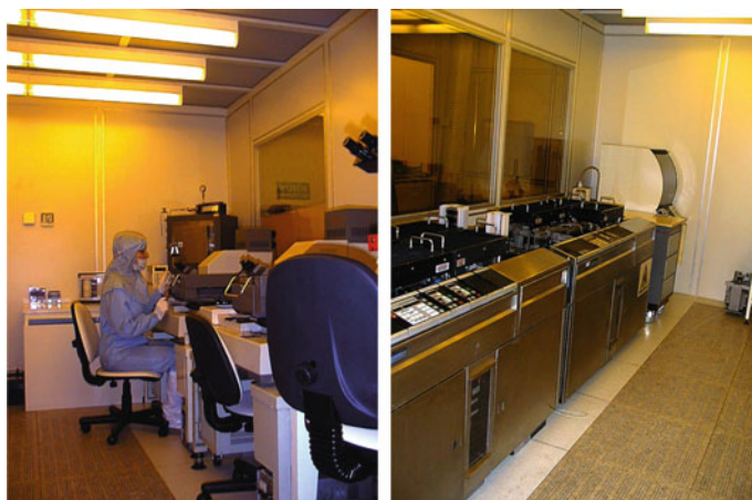
Fig. 1.56 On the left the mask-aligner is printing the mask onto the photoresist with UV light, opening the windows for the next etch process step. On the right , the spinner and developing machine can be seen. Courtesy of ITE Warsaw [347]
