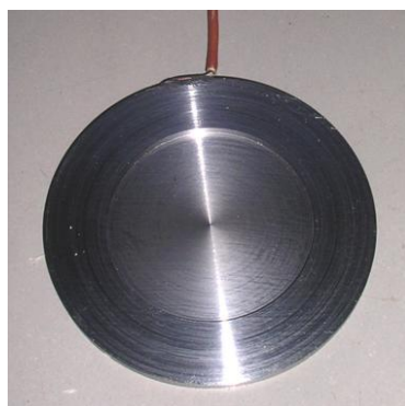
Fig. 3. Test sample after turning. The middle part is for hydrogen permeation and the machined side was in the hydrogen evolving side.
