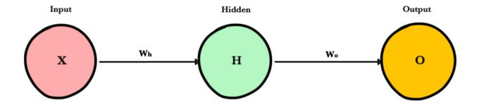
Forward propagation is how neural networks make predictions. Input data is "forward propagated" through the network layer by layer to the final layer which outputs a prediction. For the toy neural network above, a single pass of forward propagation translates mathematically to:
