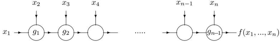
**Figure 16.** A sequence of circuits with Boolean functions  $g_1, g_2, \dots, g_n$  on a critical path  $P$ .
