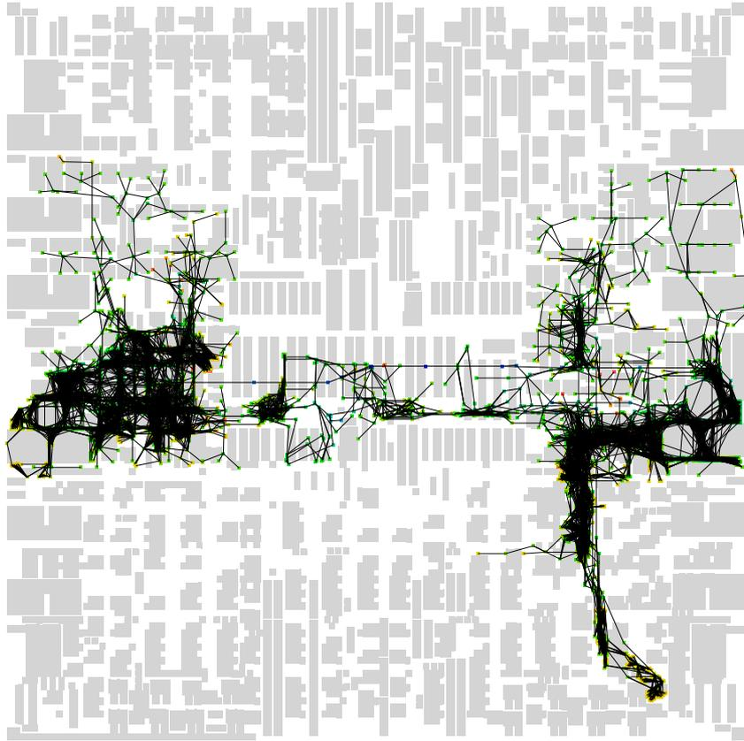
**Figure 25.** Gigahertz clock tree built by BonnClock based on the result of BonnCycleOpt shown in Figure 22. Colors indicate different arrival times as in Figure 23. Each net is represented by a star connecting the source to all sinks.
