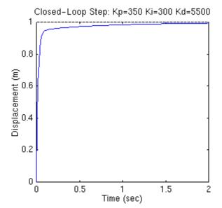
Now, we have obtained the system with no overshoot, fast rise time, and no steady-state error.
