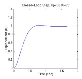
We have reduced the proportional gain (Kp) because the integral controller also reduces the rise time and increases the overshoot as the proportional controller does (double effect). The above response shows that the integral controller eliminated the steady-state error.
