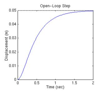
The DC gain of the plant transfer function is 1/20, so 0.05 is the final value of the output to an unit step input. This corresponds to the steady-state error of 0.95, quite large indeed. Furthermore, the rise time is about one second, and the settling time is about 1.5 seconds. Let's design a controller that will reduce the rise time, reduce the settling time, and eliminates the steady-state error.
