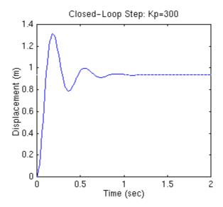
*Note*: The Matlab function called cloop can be used to obtain a closed-loop transfer function directly from the open-loop transfer function (instead of obtaining closed-loop transfer function by hand). The following m-file uses the cloop command that should give you the identical plot as the one shown above.
