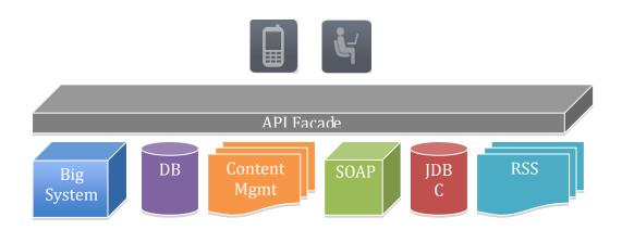
The developer and the app that consume the API are on top. The API façade isolates the developer and the application and the API. Making a clean design in the facade allows you to decompose one really hard problem into a few simpler problems.
