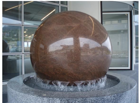
Fig. 5. The kugel fountain at the House of Science in Patras, Greece. The granite sphere has a diameter of precisely 1 m and is immersed in the water basin up to an angle  $\theta_{\text{max}} \approx 35^\circ$ . We measured the thickness of the water layer to be  $0.30 \pm 0.05$  mm.
