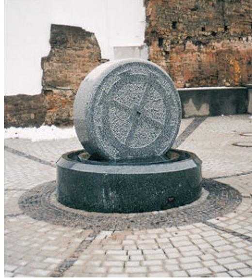
Fig. 2. A “granite wheel” fountain, in which the levitated object is a cylinder instead of a sphere. The disk in this particular fountain has an estimated radius of  $R = 0.50 \text{ m}$  and approximate width  $0.30 \text{ m}$  and is immersed in the fluid to an angle  $\theta_{\text{max}}$  of about  $35^\circ$  or  $0.60 \text{ rad}$  [cf. Fig. 3(a)].
