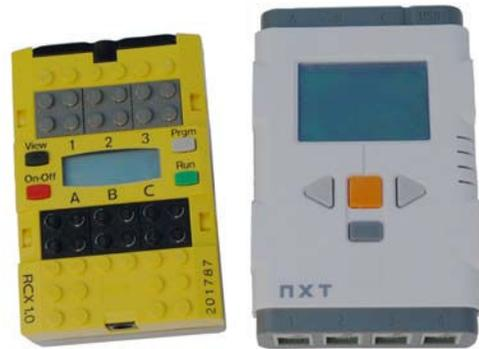
Figure 1: The RCX (left) and NXT (right) programmable bricks
