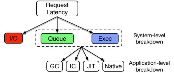
**Figure 4.** The hierarchical latency breakdown that allows us to precisely identify the bottleneck in event-driven applications.
