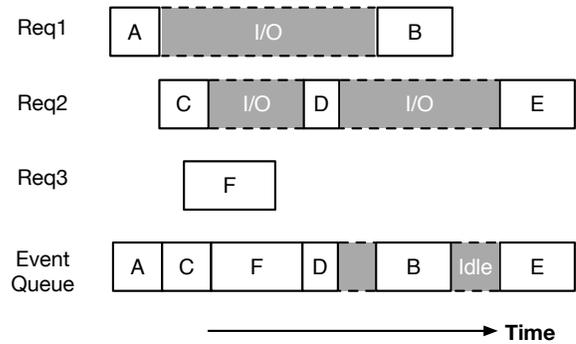
**Figure 1.** Event-driven execution overlaps compute and I/O execution. While waiting for I/O to complete for a request, the event loop is free to process events from unrelated requests. In traditional thread-per-request servers, each request is assigned a unique thread wherein a request's queue, execution, and I/O time can be directly measured. However, queue time is implicit in event-driven servers.
