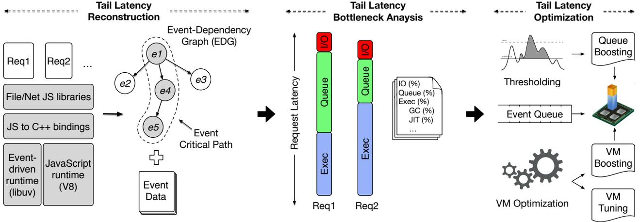
**Figure 3.** Overview of our tail analysis and optimization framework for event-driven Web services. The shaded parts indicate the components that are modified in our *Node.js*-based implementation to construct the EDG to identify request bottlenecks. The optimization stage uses the EDG breakdown to dynamically determine what optimization(s) to perform on individual requests.
