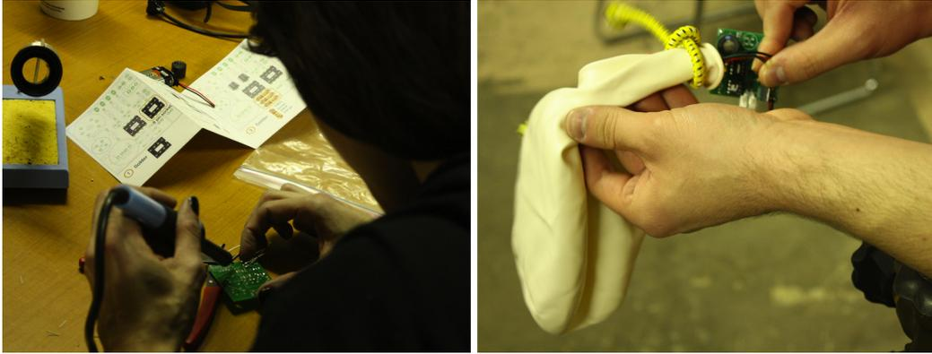
**Figure 4.5. Air quality balloon workshop: soldering components onto the PCB and attaching sensor board to the balloon.**
