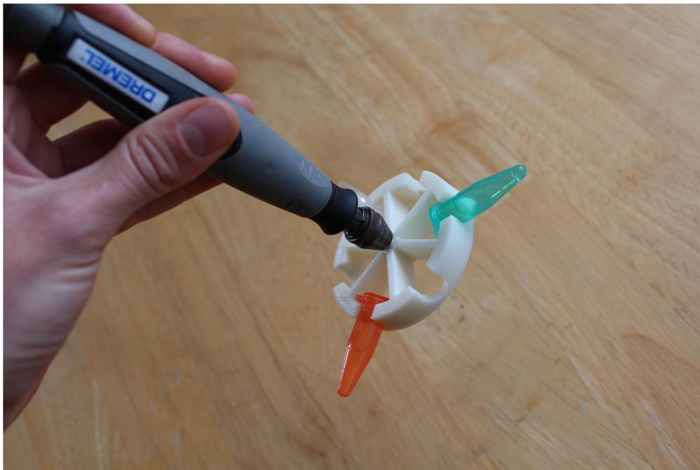
**Figure 7.2. Dremelfuge developed by Indie Biotech.**
