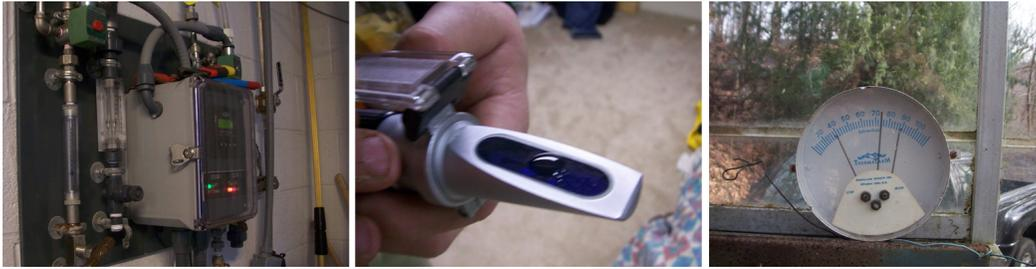
**Figure 5.2. Technologies used by participants: ORP probe, routinely used to monitor ozone levels in aquariums, refractometer, occasionally used to check honey before harvesting; thermometer, checked daily.**
