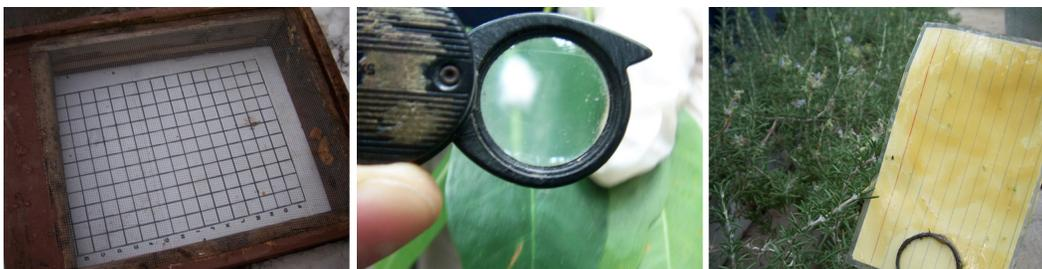
**Figure 5.3. Magnification and counting tools: monitoring tray; hand lens; handmade sticky trap.**
