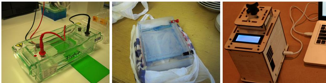
**Figure 7.3. Gel electrophoresis box in a professional lab (left) and assembled from scratch at London Hackspace (center); OpenPCR kit for replicating DNA.**
