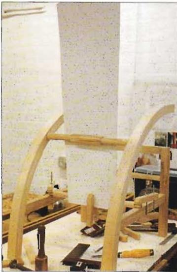
**TOP:** Adjustable bevel being used to establish backrest angle in relation to turned rails
