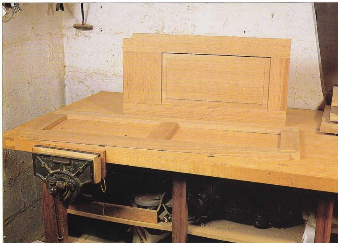
**LEFT:** Carcass sub-assemblies: side panel is tongue and grooved with a loose-fitted fielded panel; frame is mortice and tenoned – note notch for side facings
