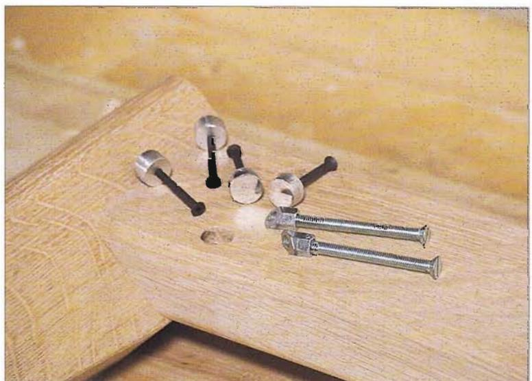
For extra security I used aluminium 4mm dowels pinned through the front and the groove at intervals down the posts. The bottom edge of the headboard is fixed to the
