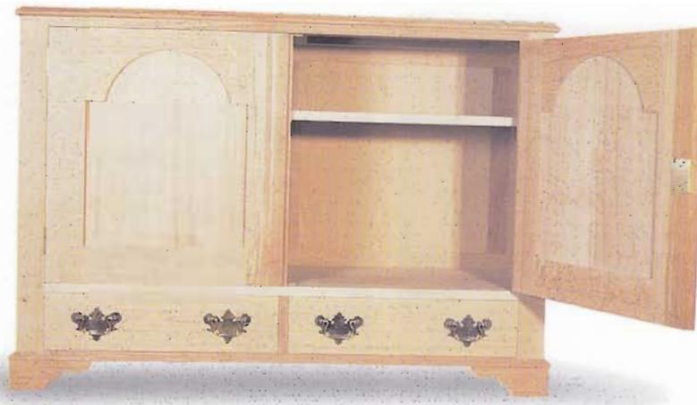
**LEFT:** Fit doors with carcass on a flat, level surface to avoid distortion
