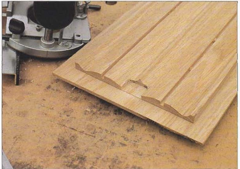
The first stage is to make a cut 7mm ( $\frac{1}{2}$ in) deep, either side of the centre line leaving a 2mm ( $\frac{1}{8}$ in) margin in the centre. A similar cut is run 5mm ( $\frac{1}{4}$ in) from each edge. Then, using the same cutter set according to the drawn shape, adjust
