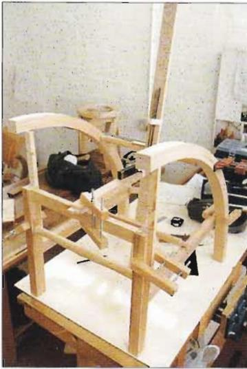
Marking out is straightforward, but care is needed in achieving the curve on the shoulders of the rear tenon on the bottom rail. This can be marked directly from the rod, *see panel*. After cutting out the joints, the front legs, front rail and seat rail can now be glued and cramped up separately.
