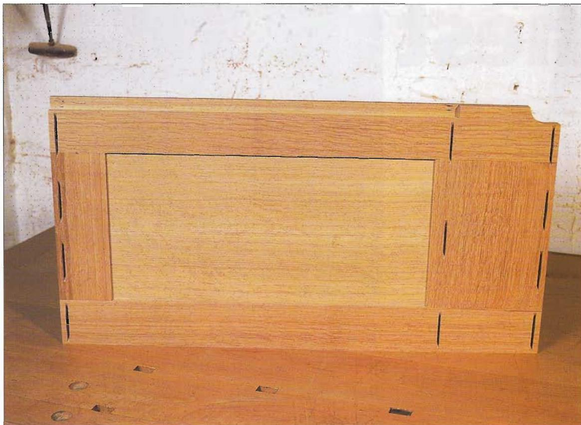
There is only one way to get a cutting list out of waney-edged English oak while obtaining the best visual effect for critical components – and that is to lay out the boards on the workshop floor and mark out the parts with wax crayon, nesting them together to avoid wastage.
