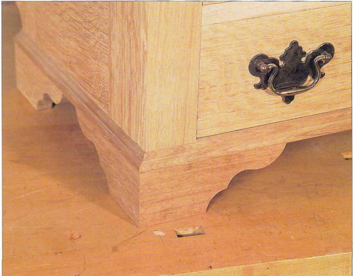
that clamps were not needed, and I still use it unless the glue pot is cold, in which case I use a fast-setting PVA such as Franklins' Wood Moulding Glue. With either adhesive the parts are rubbed into position, held briefly while the glue grabs, then left to dry.
