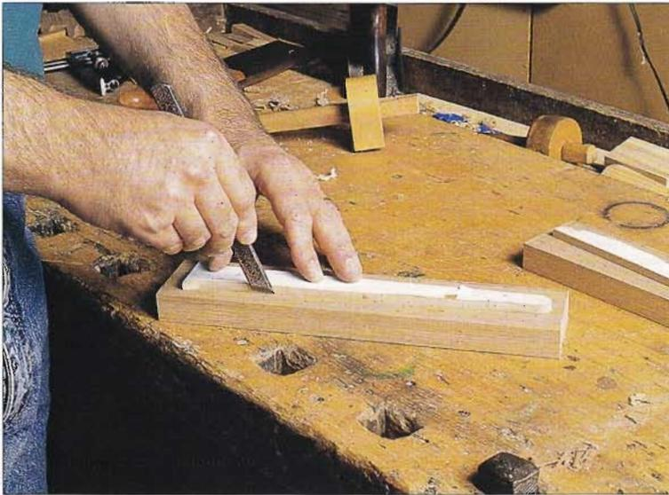
**LEFT:** Marking out the posts and feet from templates
