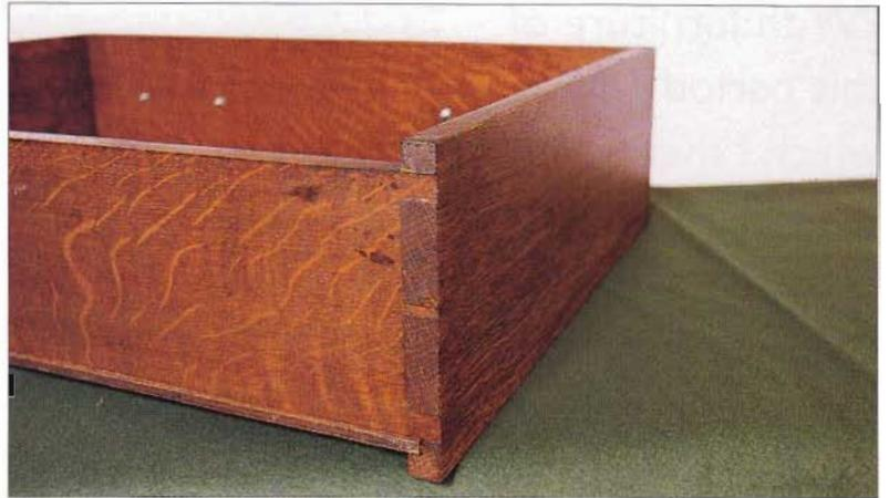
“With a chest of this kind thin, fine drawer sides look wrong and are not called for, so they are finished thick enough to be grooved for the bottoms”
