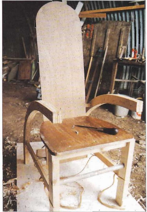
**ABOVE:** Full-size mock-up used at home to test out the practical reality of the design
