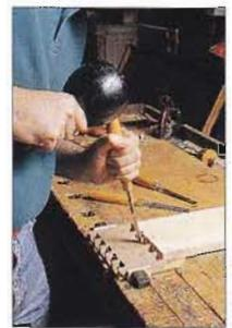
**ABOVE:** Chopping out the pins – note the angle at which the chisel is held; doing this from both faces leaves a 'hill'
