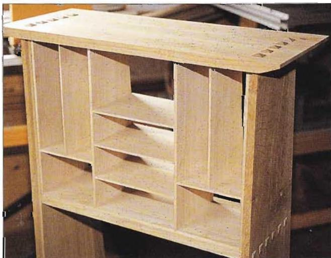
**ABOVE:** Dry-fit assembly of carcass
