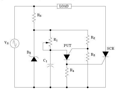
The SCR only operates on the positive half portion of the source voltage, so this is all we will deal with. When the source voltage reaches a sufficient voltage, the zener diode will begin conducting and place its voltage across  $R_1/C_1$  and  $R_2/R_3$ . The capacitor begins to charge and the PUT trigger voltage will be set to;
