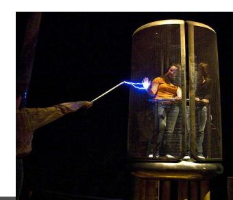
Faraday noticed that the conductor charge (on a charged conductor) did not influence anything that was enclosed within; the charge resided only on the exterior. Faraday constructed a room, coated the entire room with metal foil, and used an electrostatic generator to create high-voltage discharges that stroke the outside of his metal foil-coated room. He found no electric charge on the inside walls. Faraday used an electroscope to prove this.
