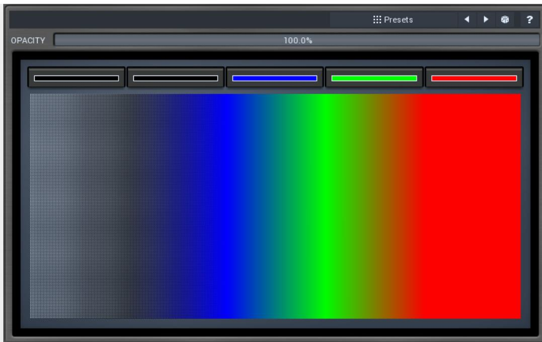
Sonogram panel contains visual settings of the sonogram, mainly the sonogram colors. A sonogram uses a set of colors. When the particular frequency's level is minimum, the first color is used. When it is maximum, the last color is used. Otherwise it interpolates colors in between.
