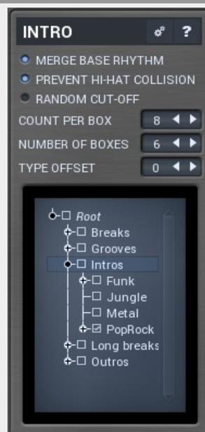
Intro panel provides configuration of generator parameters for intro loops.
