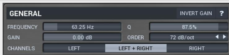
General panel contains standard filter settings such as frequency or Q. Most of these values are available directly from the band graph, but it may be necessary to use these controls for more accurate or textual access.
