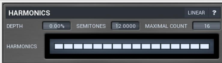
Harmonics panel contains parameters of harmonics - cloned bands created at defined higher frequencies. This is often useful to remove natural noises, which usually bring some harmonics with them etc.
