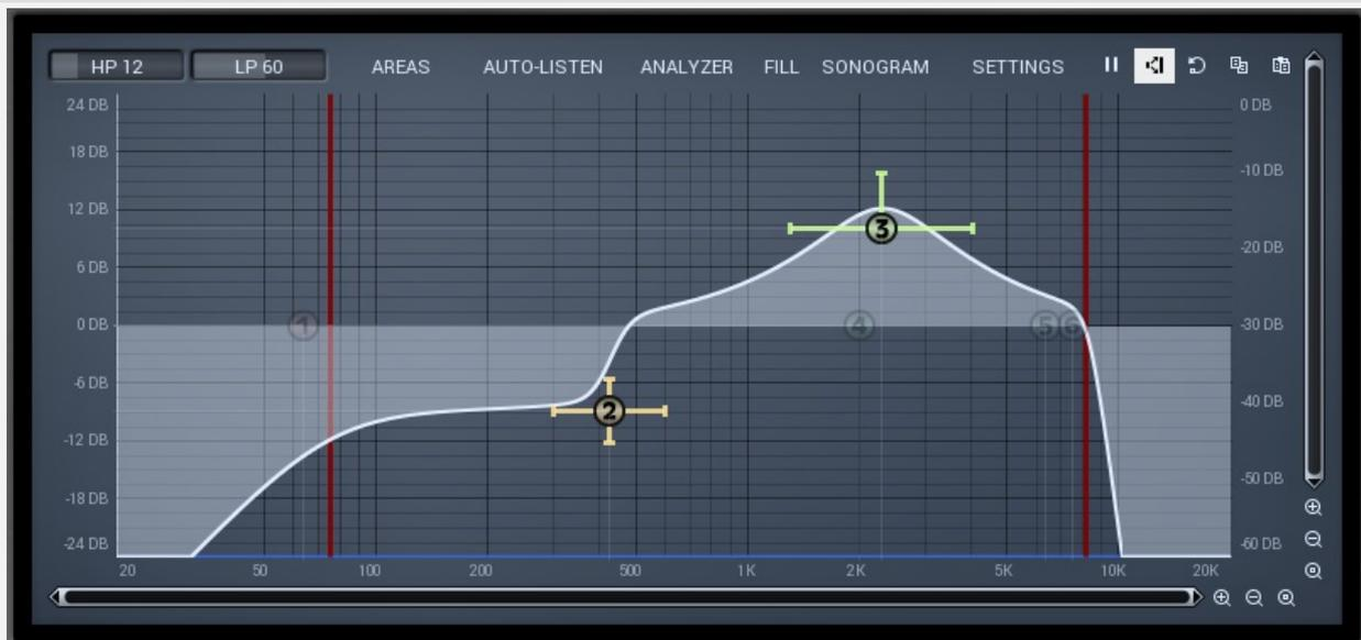
Equalizer shape graph controls the frequency response. There are several bands available, each of them can be enabled/disabled, can be set to a different filter, can have different frequency, Q and other parameters. Double-click on a band point to enable or disable a band. Drag it to change its frequency and gain. Drag the horizontal nodes to change its Q. Hold **ctrl** key for fine tuning. Click using the right mouse button on it to open a window with additional settings.
