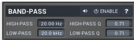
Band-pass panel contains parameters of the band pass, which you can use to additionally process the signal used measure level of the band. For example, you may want a band at high frequencies react to bass content by placing the band anywhere on the high frequencies and set the low-pass at say 200Hz.
