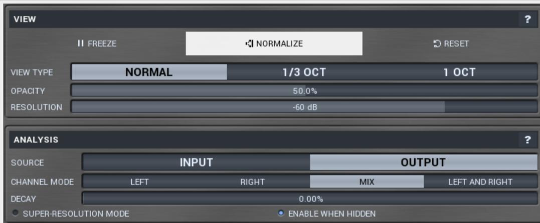
Main settings panel contains the most useful settings controlling the analyzer behaviour and view.
