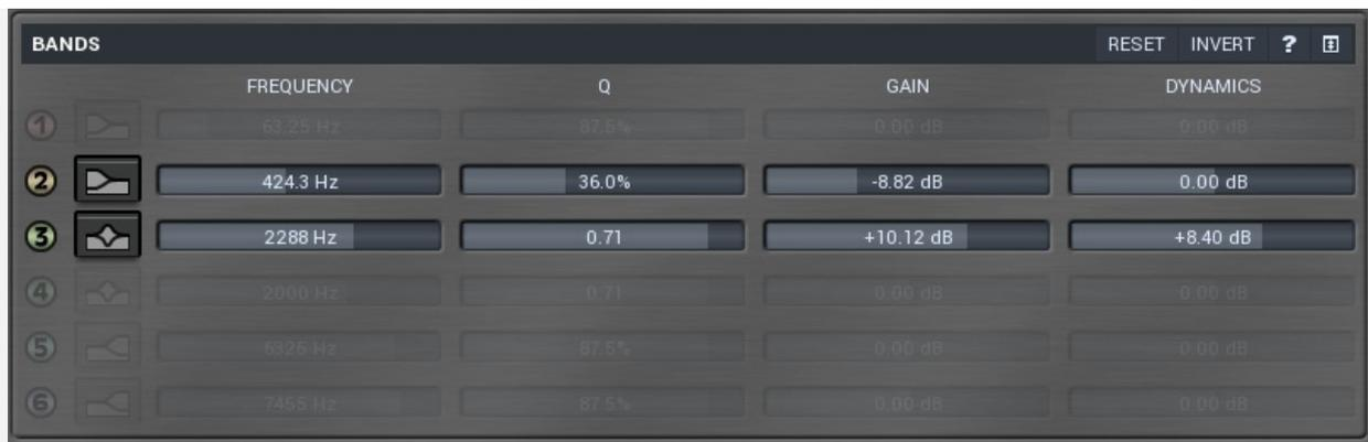
Bands panel contains the list of available bands along with their basic parameters. You can use it to enable/disable a band, change the parameters and show the settings window if you don't like editing the bands from the equalizer panel or if you need to set some values by text. The panel is collapsed by default, because it takes lots of space.
