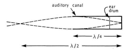
The natural frequency for an air-filled tube of length L with one end closed is:
