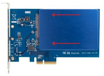
2 Slide the SATA connector on the drive into the SATA connector on the Accelsior S. Ensure the drive is fully seated, as shown.
