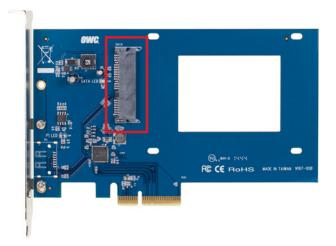
1 Set the OWC Accelsior S down on a flat surface. Make sure the black SATA connector is facing up, as shown above.
