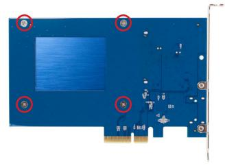
Install the four Phillips screws into the four screw holes to secure the drive to the Accelsior S, as shown.
