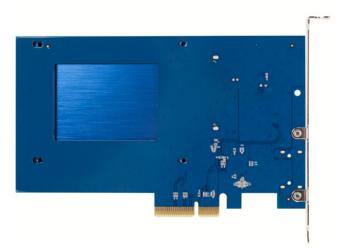
3 Holding the drive securely to the Accelsior S, turn over the Accelsior S.
