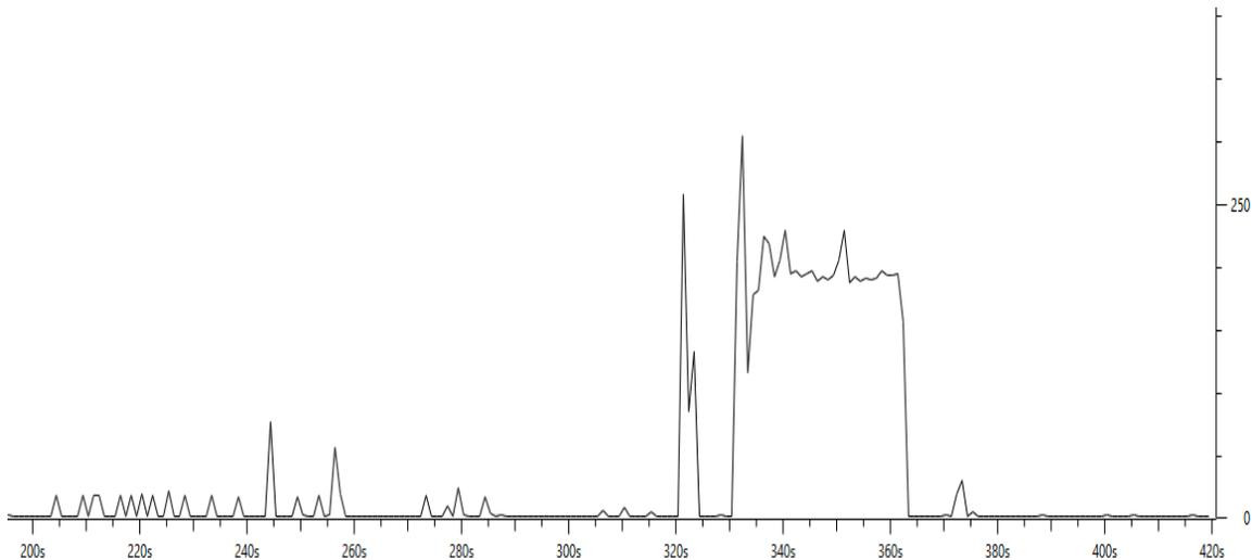
Figure 10: Sample Network I/O Data from a Malicious Firmware Update to an Industrial Ethernet Switch<sup>37</sup>
