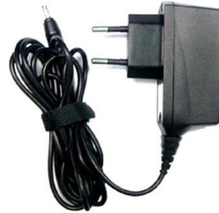
*External power supplies are either AC-AC (convert AC input to a lower voltage) or AC-DC (convert AC input to DC output). They are physically separate from the device they power and connect to it with a cable.*
